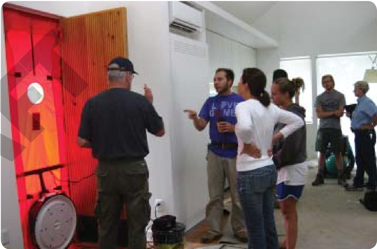
Bruce Glanville, LEED Green Rater, conducts blower door test on home. Test results revealed only .04 natural air changes/ hour. (above)
