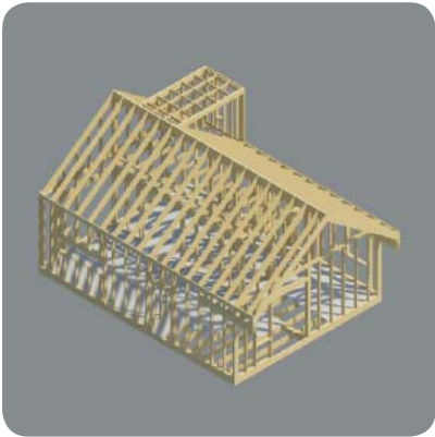
Modular units are set on-site 24" O.C. roof joist spacing (top-left)
